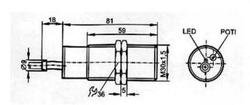
The sensor is adjusted at the factory for most materials. If the unit does not load material and the sensor light is not lit, turn the adjustment screw on the back of the sensor counterclockwise until the light is lit. If the loader does not stop loading with material in front of the sensor, turn the adjustment screw (POT1) clockwise until the light goes out. The adjustment screw has a 20-turn adjustment with
